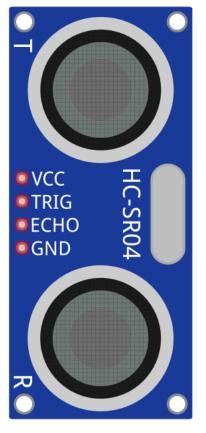
**Note:** The output voltage of the module is in the 5V range. In order to use the module with the Raspberry Pi, the device called logic level converter should be used. Otherwise connecting 5V signals to the GPIO pins may cause damage to the Raspberry Pi. For this purpose use the device called *TXS0108E Logic Level Converter* that AZ-Delivery offers.
