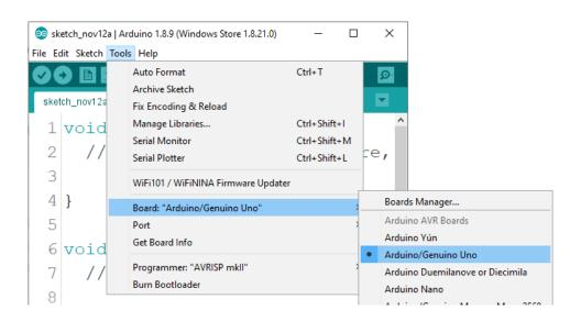
The port to which the Arduino board is connected has to be selected. Go to:
