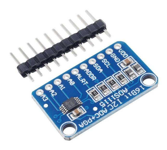
The ADS1115 module is a four channel breakout board. These modules are perfect for adding high-resolution analog to digital conversion to any microprocessor-based (like Raspberry Pi) project or if you want to add analog to digital converter with higher accuracy to and microcontrollerbased (like Arduino) project.
