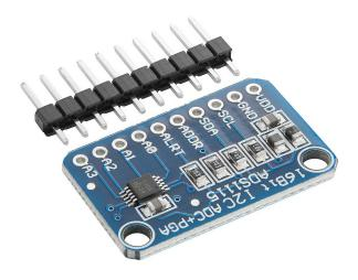
The Raspberry Pi is not able to read analog voltages because it does not have an analog to digital converter. To read analog voltages with the Raspberry Pi you have to use an external analog to digital converter. The AZ-Delivery offers this kind of device, it is called *ADS1115 Analog to digital converter*.
